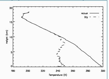
Figure 3. A depiction of cold bias in "dry" temperature below 10km Realistic temperature and pressure profile require inclusion of water vapor pressure (e) term in equation (7) and (10) for retrieval below 230K. This
