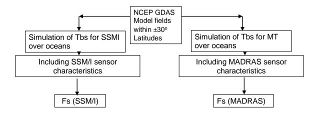
Fig. 2: Scheme for simulation of brightness temperatures for SSM/I and MADRAS using NCEP environment fields and finding regression relation for expected brightness temperature at 85.5 GHz (SSM/I) / 89 GHz (MADRAS).
