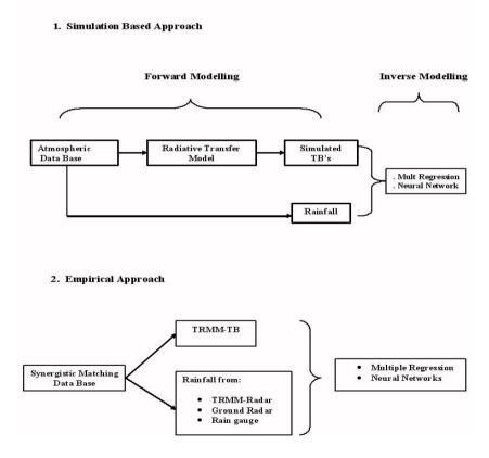
Fig. 2 Flow Diagrams showing the Concept of Rainfall Retrieval:
