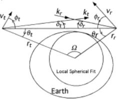
Figure 2. Occultation geometry defining the angles used in equations 2(a, b).
