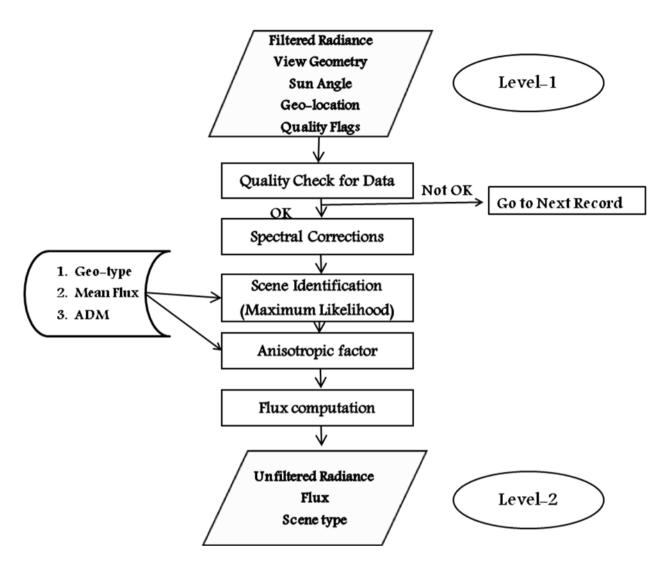
Fig. 2: Flow chart of Level-2 data processing system.
