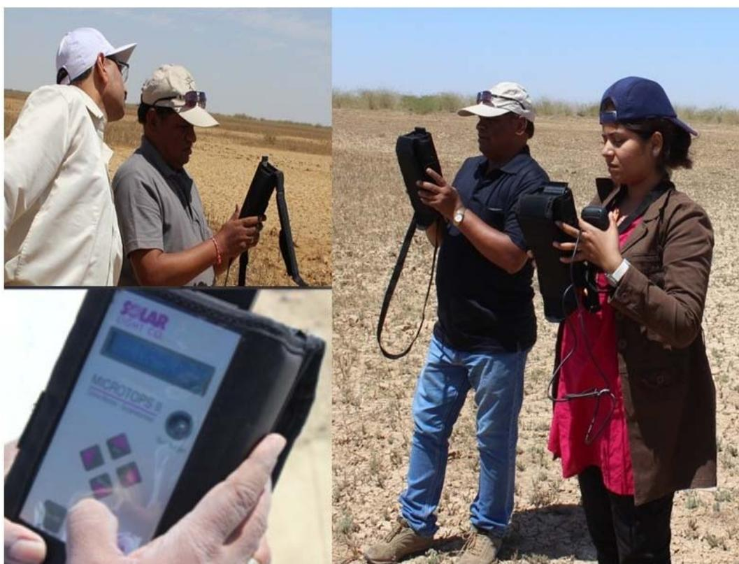
**Figure 5:** Measurements of atmospheric parameters (aerosol optical depth, total columnar ozone and water vapour) using MicroTops-II sunphotometer and ozonemonitor during the campaign
