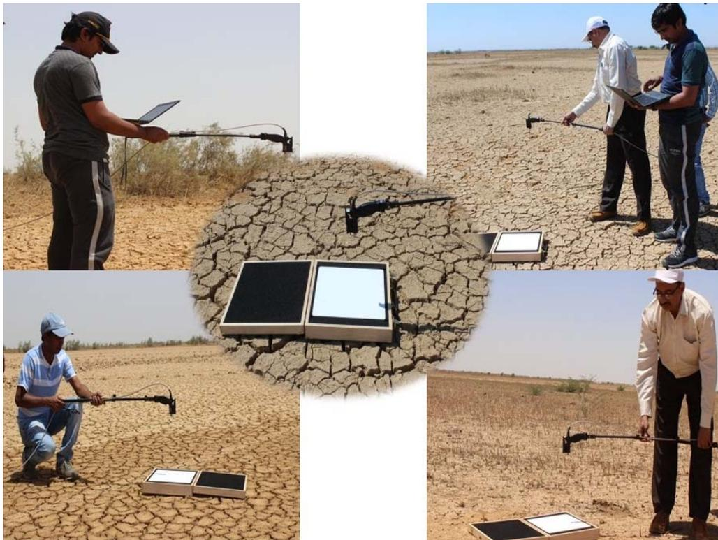
**Figure 4:** Collection of surface reflectance using ASD hyper-spectral radiometer during the campaign
