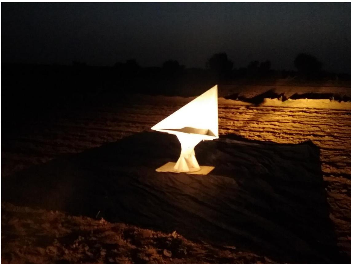
Figure 5-46 CR deployed on black cloth background
