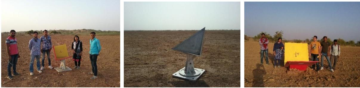
(e): Deployed Corner Reflectors
