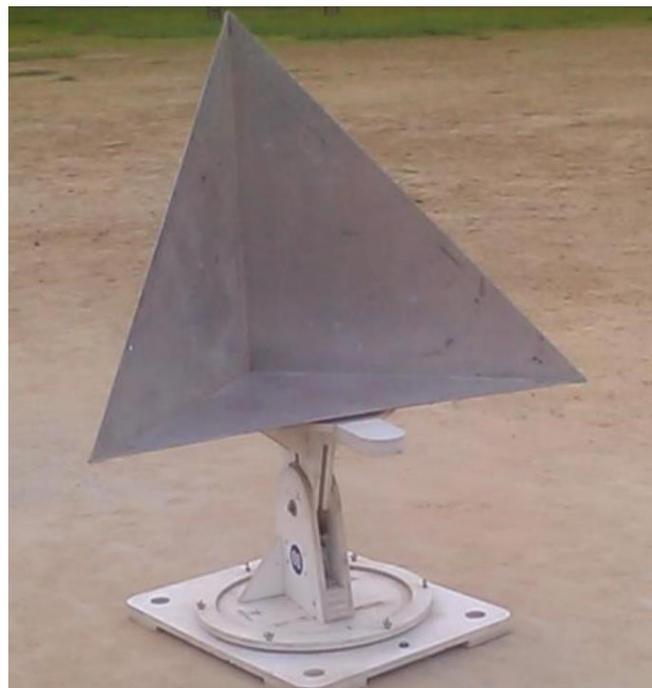
**Figure 3-1 Triangular Trihedral Corner Reflector (size 0.90m)**
