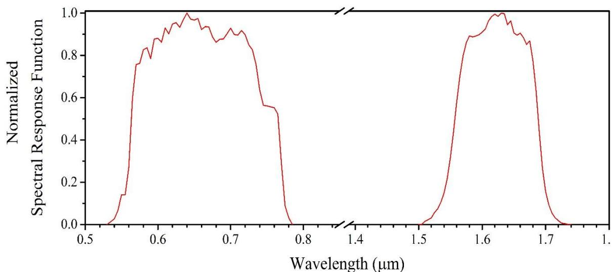
*Figure 4: Pre-launch laboratory measurements of spectral response function for VIS and SWIR bands of INSAT-3DR*
