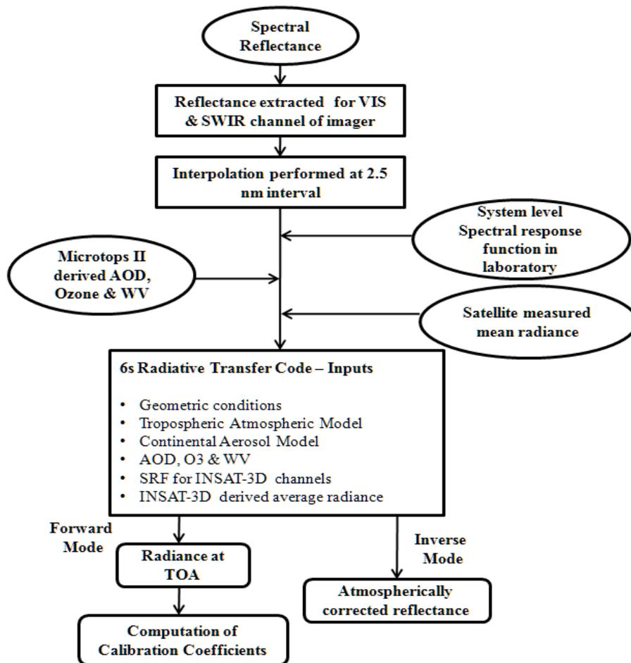
*Figure 6: Flow chart for the simulation of TOA radiance and estimation of calibration coefficient.*
