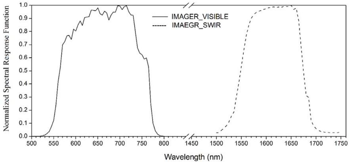
*Figure 8: Pre-launch laboratory measurements of spectral response function for VIS and SWIR channels of INSAT-3D.*
