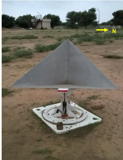
Figure 6: Trihedral Corner reflector deployed in Bopal cal-val site
