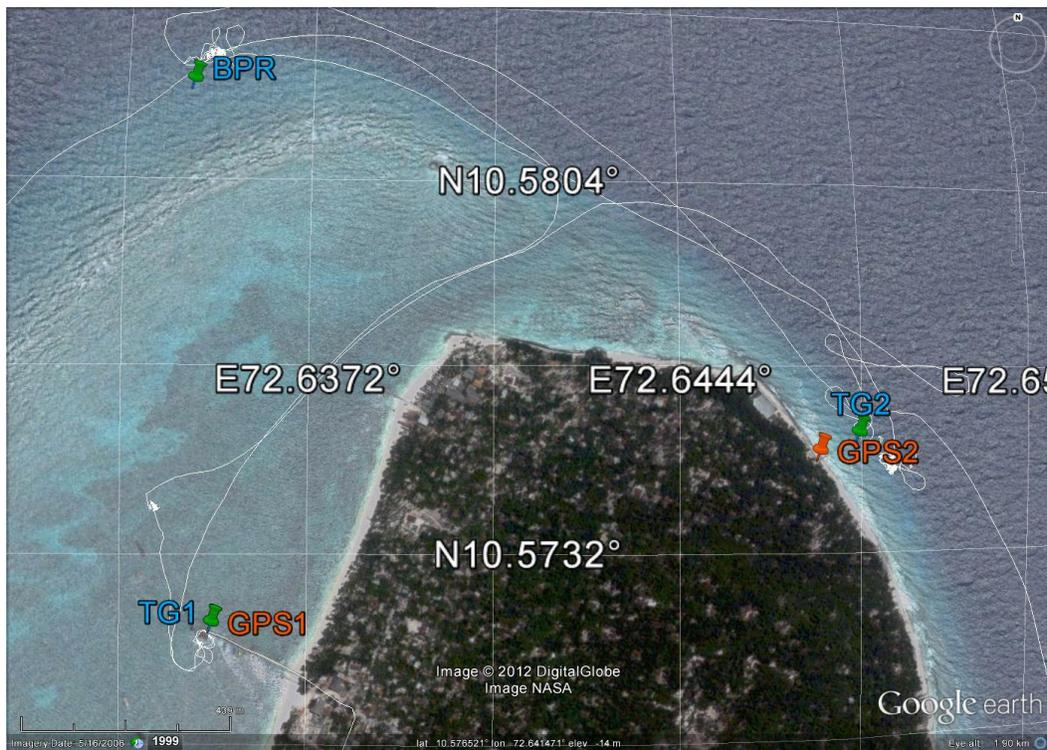
**Figure 9:** Positions of the instruments at main Jetty (GPS1 and TG1), at NIOT Jetty (GPS2 and TG2) and at offshore BPR mooring. The white track displays the temporal positions of the GPS buoy.
