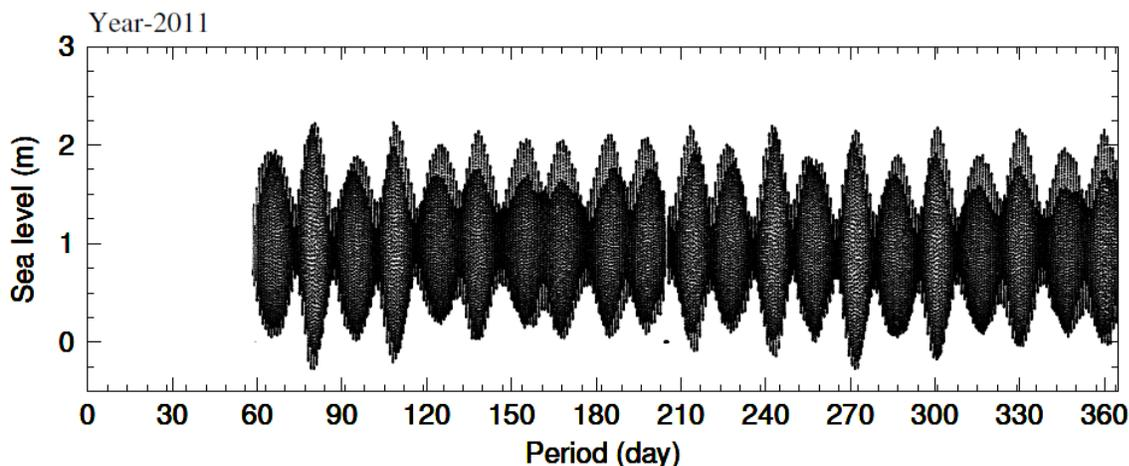
**Figure 4b:** Time series tidal observations from Port Blair tide gauge for the year 2011
