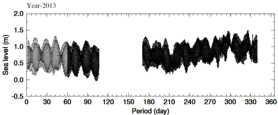
**Figure 6b:** Time series tidal observations from Machlipatnam tide gauge station for the year 2013.
