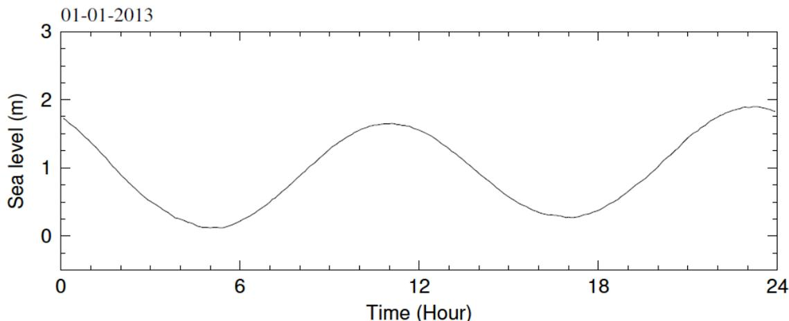
**Figure 4a:** One day tidal observation from Port Blair tide gauge station.
