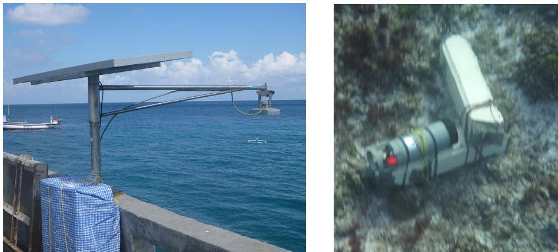
**Figure 10:** Downlooking aerial microwave radar gauge at NIOT jetty (right panel), the bottom pressure recorder at deployed condition at off lagoon Kavaratti (left panel).
