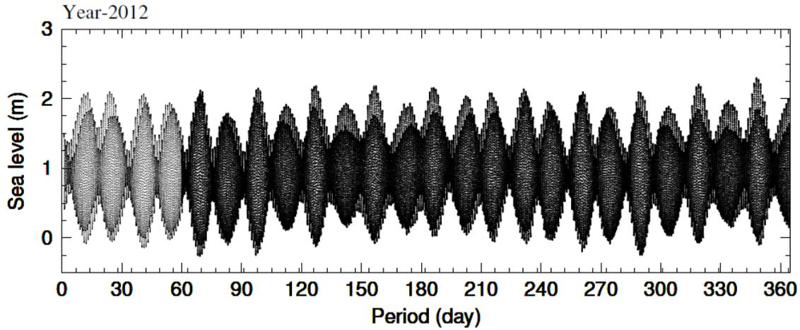
**Figure 4c:** Time series tidal observations from Port Blair tide gauge for the year 2012
