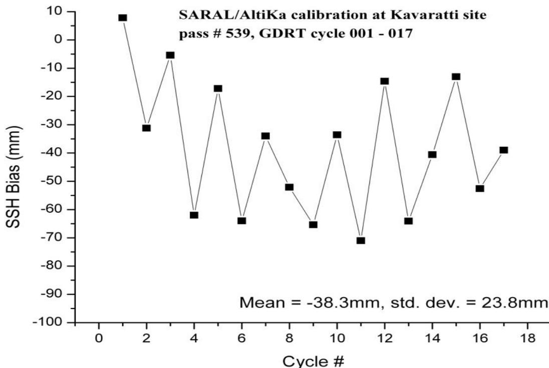
**Figure 22 :** SARAL/ALtiKa SSH bias from cycle 1 to 17 using GDR-T products.
