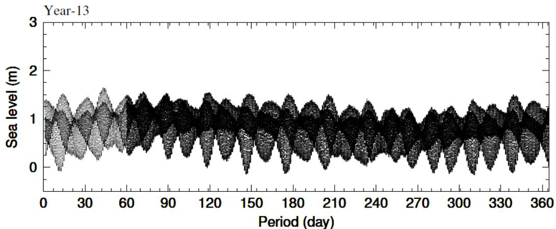
**Figure 8b:** Time series tidal observations from Kavaratti NIOT jetty (TG2) tide gauge station for the year 2013.
