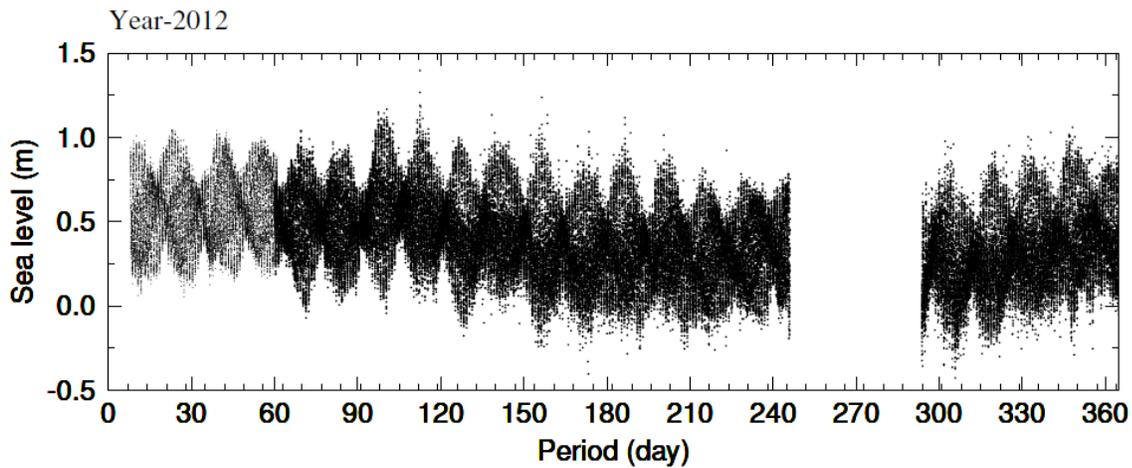
**Figure 5a:** Time series tidal observations from Kanyakumari tide gauge station for the year 2012.
