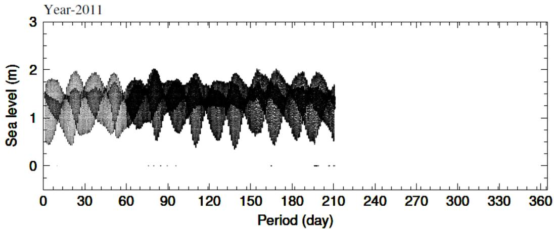
**Figure 7b:** Time series tidal observations from Kavaratti main jetty (TG1) tide gauge station for the year 2011.
