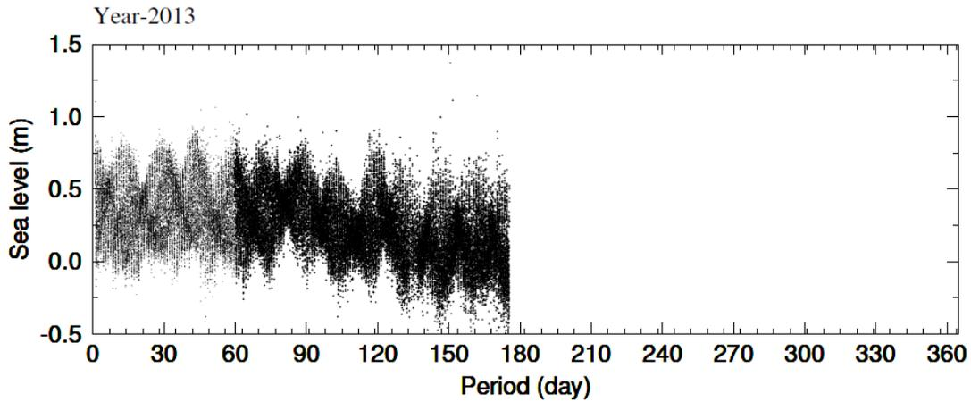
**Figure 5b:** Time series tidal observations from KanyaKumari tide gauge station for the year 2013.
