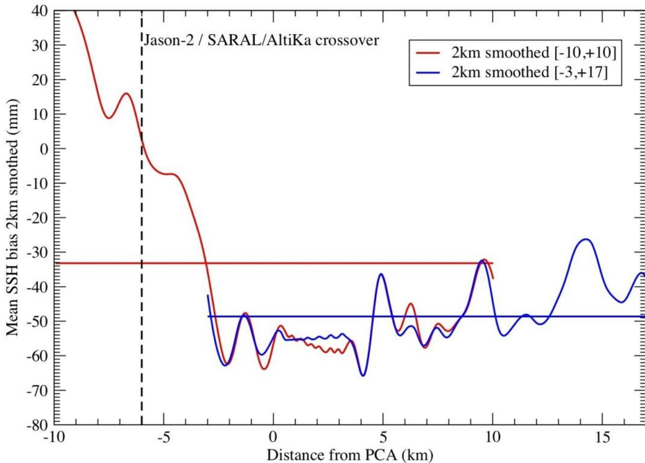
**Figure 21:** SARAL/ALtiKa SSH bias as a function of distance from the PCA
