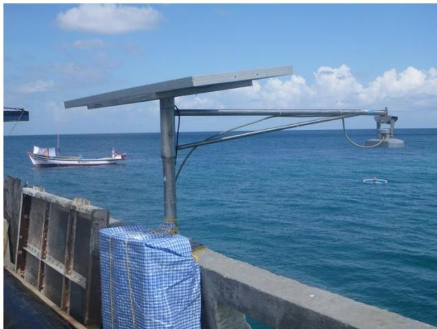
**Figure3:** Typical installed radar gauge at Kavaratti site
