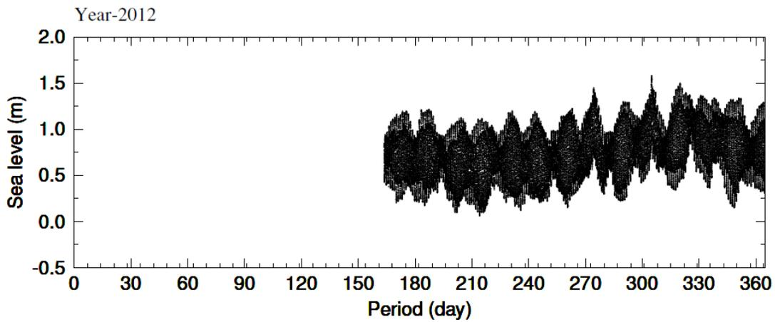
**Figure 6a:** Time series tidal observations from Machlipatnam tide gauge station for the year 2012.
