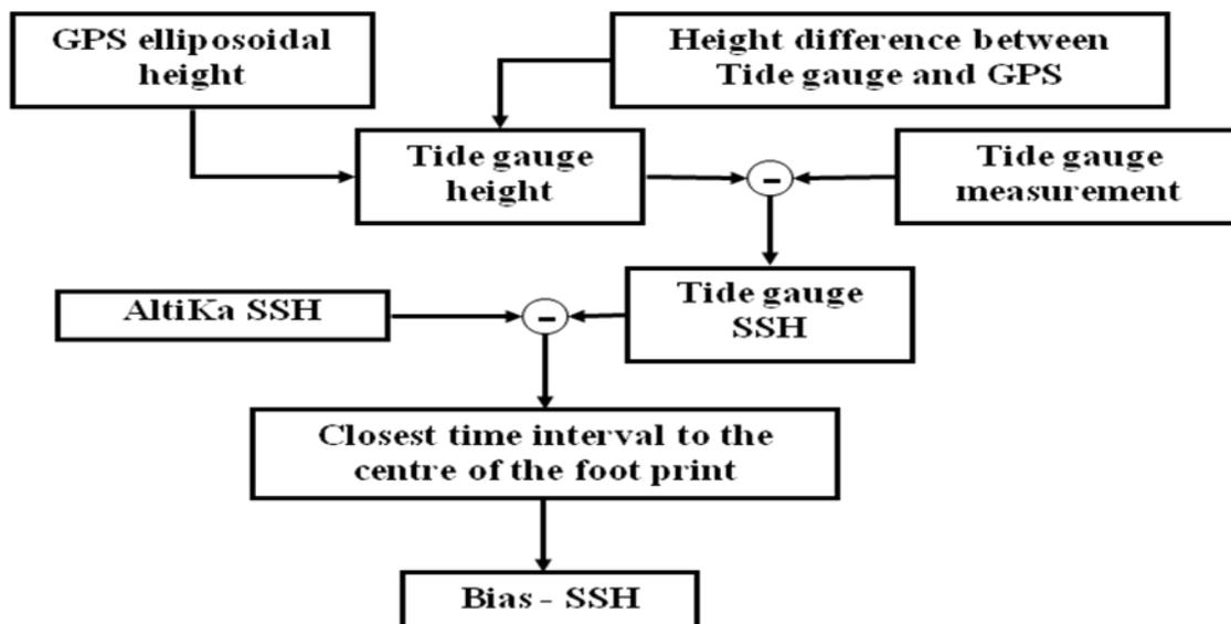
**Figure 20:** Flowchart of absolute SSH calibration of altimeter user tide gauge observations.
