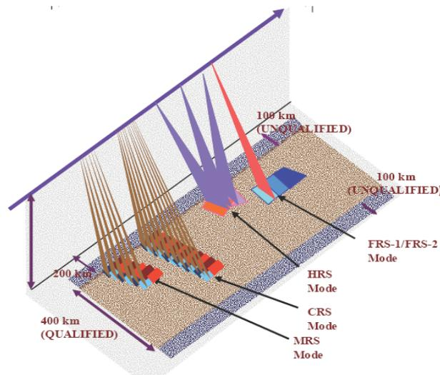
**Fig.1:** Schematic Diagram showing different beam modes of RISAT SAR
