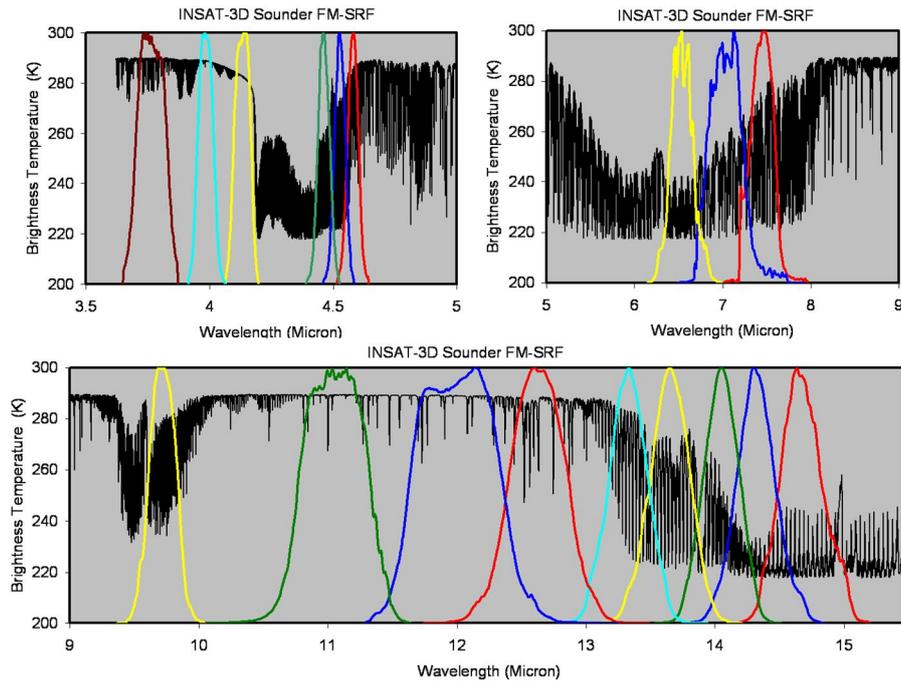
*Fig.2a: INSAT-3D Sounder SRFs overlaid on IASI spectrum*
